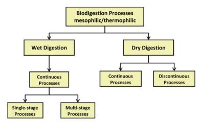
Fig. 3 Types of anaerobic treatment technologies and processes
