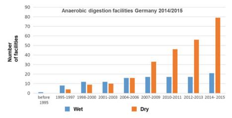
Fig. 4 Years after starting the operation of anaerobic treatment facilities for biowaste and green waste
