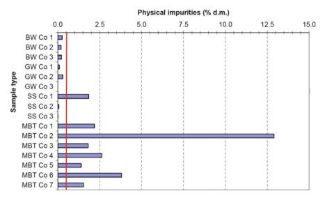
Fig. 2 Physical impurities (glass, metal, and plastic particles >2 mm) in compost samples collected by JRC and sent by plants
