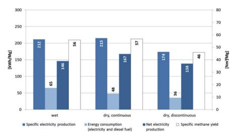
Fig. 5 Comparison of electricity production, consumption, and net electricity yields of wet and dry processes for anaerobic treatment of biowaste and green waste relative to the input into the facility
