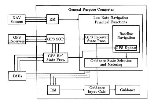
Fig. 1. Architecture for integrating GPS into navigation subsystem.
