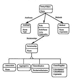
Fig. 5. An integrated data model for OOA/D and EER modelling.
