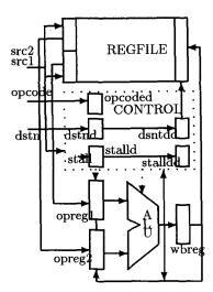
Fig. 1. A Pipelined Microprocessor
