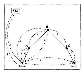
Fig. 5. Authentication with globalized keys
