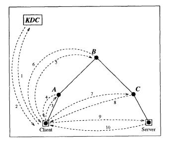
Fig. 4. Authentication with localized keys
