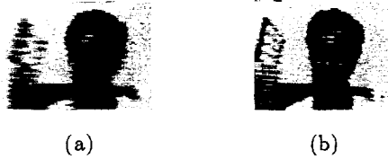
Figure 12. 32 pixels by 32 pixels 5% filtered Head & Shoulder pictures. (a) A Raster Scan's picture. (b) A SFC Scan's picture.
