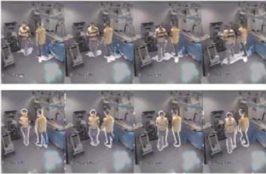
Fig. 7. (Sequence 2) An image sequence showing two people walking towards each other inside an operating theatre. Results of object identification based on background removal (top) and neuro-fuzzy filter (bottom), respectively
