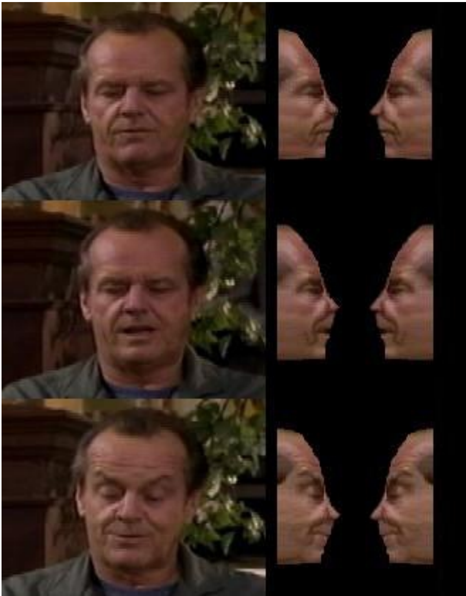
Fig. 5. Video frames with profile views synthesized from a structure-from-motion analysis of the 70 \times 80 pixel facial region. The profiles are mirror images except for differences in recovered 3D structure. The profiles on the left have poor structure between the mouth and nose because occlusion artifacts in the tracking were correlated with head nods. The profiles on the right have better shape from the tip of the nose to the top of the mouth because incomplete SVD was used to handle occlusions in the 3D reconstruction.
