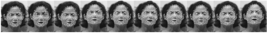
Fig. 4. Every 300th frame from a 3000-frame sequence tracked via rank-constrained optical flow with incremental SVD. Dots are superimposed on the video by the tracker.
