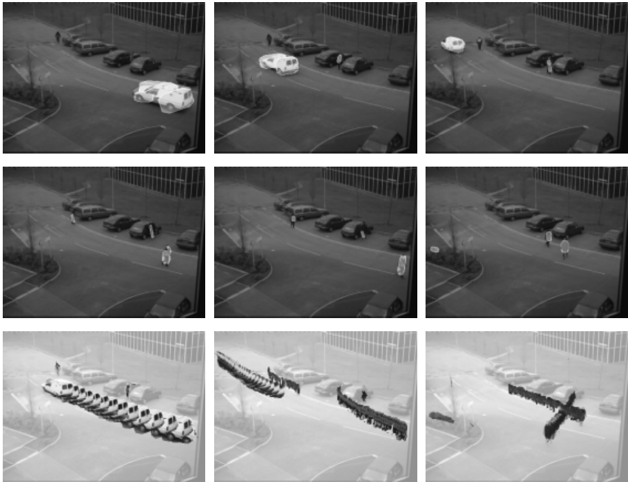
Fig. 5. The optimal models found for the PETS2000 sequence, (top) frames 802, 842, and 882, (middle) 1002, 1042, 1202. The car, three pedestrians, and bushes blowing in the wind (middle-right) are detected. (bottom) Composite images formed from all the polybones of the optimal models in every fourth frame, for frames (bottom-left) 750 to 850, (bottom-middle) 850 to 1070, and (bottom-right) 1070 to 1290. Note that the car and the pedestrians are consistently detected.
