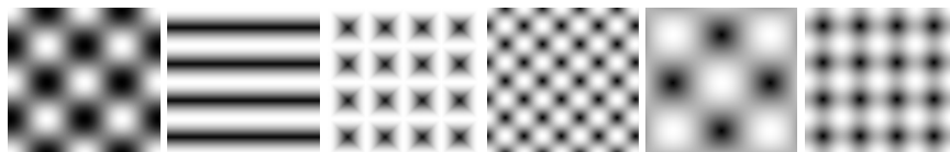
Fig. 1. Symmetries of the odd filters obtained from the considered quadrature approaches. From left to right: the partial Hilbert transform with preference direction \mathbf{n} , the total Hilbert transform, the three imaginary components of the quaternionic analytic signal, and the Riesz transform (vector valued)
