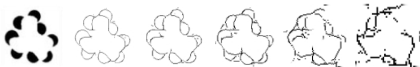
Fig. 7. A synthetic image and the outputs of a single-scale contour completion algorithm on this image at different sizes. The figures correspond to completion over increasingly coarse scales.
