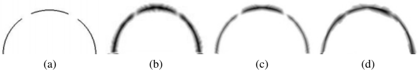
Fig. 9. A synthetic example of the use of multi-scale conditioning. (a) the original input. (b) the completion at the coarse scale. (c) the completion at the fine scale without using the conditioning in Equation (13). (d) the completion with the conditioning.
