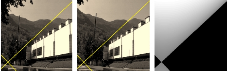
Fig. 7. A pair of images of the Grenoble museum from which one wishes to compute the focal lengths. It is assumed that the principal point \mathbf{p}_1 in the first image is the centre of the image. Shown overlaid on the first (left-hand) image are the epipolar line [\mathbf{e}_1] \times \mathbf{p}_1 and the perpendicular epipolar line [\mathbf{e}_1] \times \mathbf{I}[\mathbf{e}_1] \times \mathbf{p}_1 . Overlaid on the second (right-hand) image are the corresponding epipolar lines \mathbf{F}\mathbf{p}_1 and \mathbf{F}\mathbf{I}[\mathbf{e}_1] \times \mathbf{p}_1 . From these latter two lines one may compute the focal length f_2 . Computation of the focal length f_2 will be very imprecise in this case, since the angle \theta between these two lines is close to 90^\circ , and also because one of the lines (actually \mathbf{F}\mathbf{p}_1 ) passes very close to the centre of the image, and hence (presumably) close to the principal point \mathbf{p}_2 . Relative accuracy of the focal length f_2 is given by (3), and is proportional to the distance of \mathbf{p}_2 from each of these two epipolar lines, and also to the tangent of the angle \theta .
