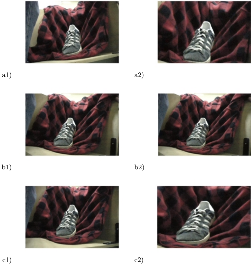
Fig. 3. Using the computed homographies through the planes at infinity to generate a virtual motion of pure translation. Figures b1,b2 contain the same image, to which the input images were warped. Figures a1,c1 to the left are the original input images. Figures a2,c2 to the right are the results of warping a1,c1 by the respective homographies through the plane at infinity.
