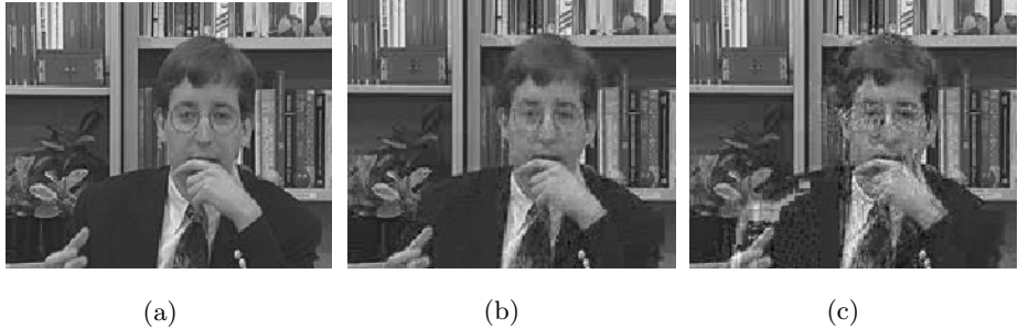
Fig. 2. Original frame 2(a), source-coding distortion 2(b), and source-coding plus channel distortion 2(c).
