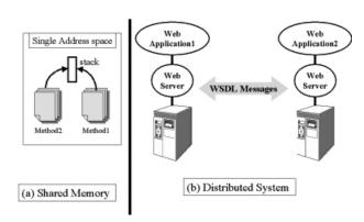
**Fig. 7.** Schematic of two bindings of a Web Service (a) Single address Space and (b) Distributed
