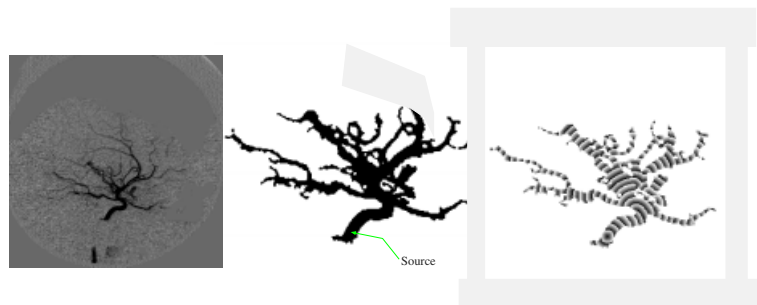
Fig. 6. Application of the geodesic labelling in medical imaging: left An angiography image, middle binary image when blood vessels are segmented and right the geodesic labelling.
