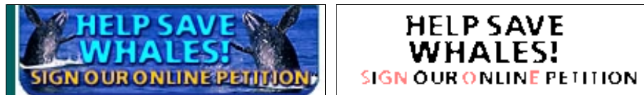
Fig. 9. An image containing single-colour characters over multi-coloured background and the corresponding results
