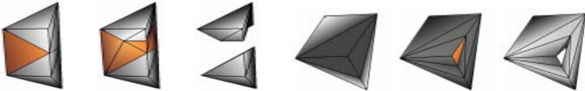
Fig. 6. Removal of an edge(left) and of a vertex(right) singularity after an optimized local refinement
