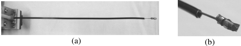
Fig. 3. The Flexible Drilling Unit : (a) overview: 250 mm in length and 3.5 mm in diameter (b) the end-mill on the tip of the unit: It rotates and vibrates axially. Graft is harvested from an aperture between flexible tube and the rod of the end-mill
