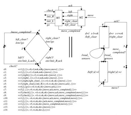
Fig. 1. Example system with robot M1 and controller M2 with possible computation sequence at bottom left.
