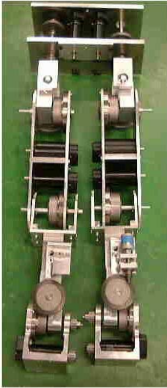
Fig. 2. The mechanical design and a photo of the lower part of KENSEI-chan
