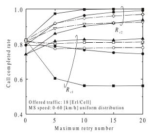
**Fig. 4.** Call-completed rates versus maximum retry number.
