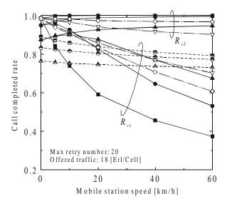
Fig. 3. Call-completed rates versus MS speed.
