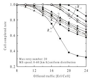
Fig. 2. Call-completed rates versus traffic load.
