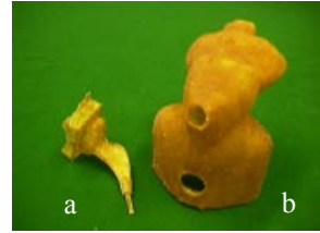
Fig. 10. a) The latex skin for the original cavity. b) The latex bladder which contains the gelatine phantom. Note the large hole at the bottom to allow ultrasound scanning.
