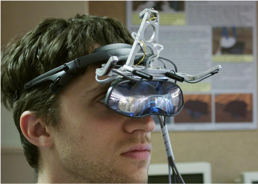
Fig. 2. Video-see-through augmented reality HMD built on the basis of a Sony Glasstron LDI-D100 device. The aluminum superstructure holds two miniature video cameras for image capture and three infrared LEDs for opto-electronic tracking of the HMD
