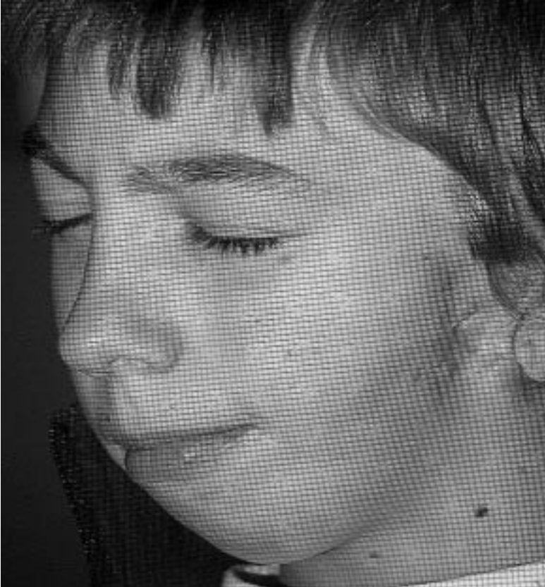
Fig. 2. For the acquisition of 3D photographs structured light is used, projecting a pattern onto the face. 3D structure can be extracted from the deformation of this pattern.
