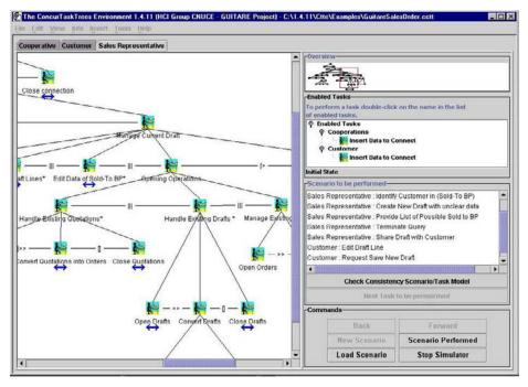
Fig. 2. Example of Abstract Scenario Derived from Task Model
