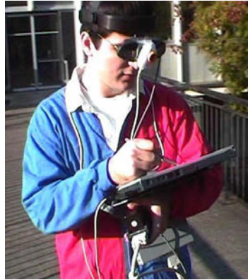
Fig. 2. A MAGIC user, equipped with the HMD and holding the pen computer
