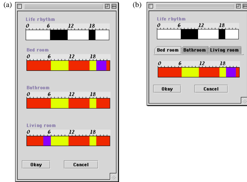
Fig. 1. a) Large screen. The temperature of the rooms are available at a glance. b) Small screen. The temperature of a single room is displayed at a time.
