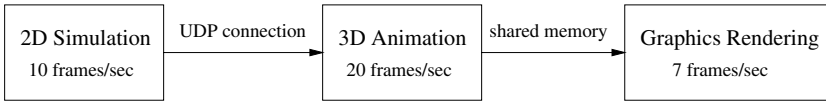
Fig. 7. The animation process generates 3D scenes at a fixed rate of 20 frames per second. In the experimental setup, a rendering speed of 7 frames per second was achieved. This information loss might contribute to the insignificant effect of kick animations on perceived playing skill.
