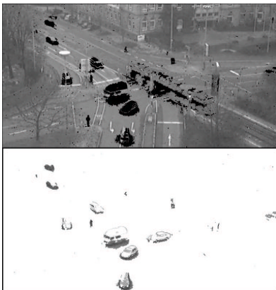
Figure 3: The upper image shows a recall of frame 0400 using background cells learned from frame 0000. The lower image is the resulting motion segmentation at frame 0400 achieved with the Algorithm 2.
