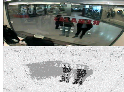
Figure 5: Frame 0569 from the third testing video sequence of the PETS2002 dataset [2] (above). Below its representation using cells computed by Algorithm 3. Light grey is used for cells from the background layer, darker grey for the dynamic and black for the static object layer.
