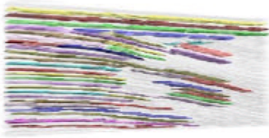
Fig. 4. 40 largest horizons which resulted from the merging process obtained with the parameters shown in the last row of table 1.
