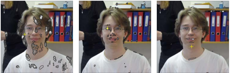
Fig. 1. The likelihood fields in sample images. Manually selected location of the features are marked as + in the images. There are multiple false matches in all the images, and the maximum likelihood for the chin point occurs in an incorrect location, as due to lighting the chin shadow is almost non-existent.
