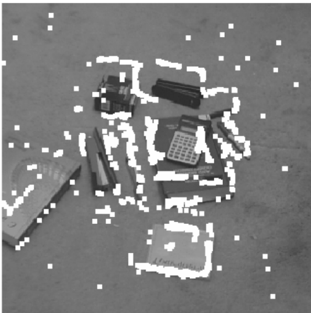
Fig. 2. The failure of the “simplistic” detectors, depicted in Fig. 1, to correctly locate the pocket calculator. Detection is marked by a small bright square at the upper left corner of the detected image region. Not only are there many false alarms, but the correct location is not detected. In the sequel, it will be shown that very accurate detection can be achieved by using better detectors.
