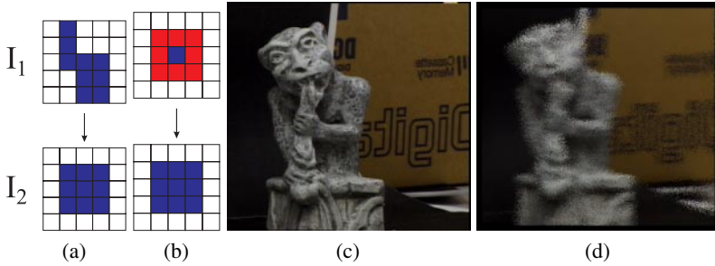
Figure 1. Shuffle transformations. (a) A 1-shuffle corresponding to a piecewise-continuous image translation. (b) A 1-shuffle corresponding to a non-parametric image transformation; this example shows that r -shuffles can model the process of “ignoring” a subset of the pixels in an input image. (c),(d) A randomized 10-shuffle: the image in (d) was created by displacing every pixel in (c) to a randomly-selected position inside a 21 \times 21 pixel window centered at the pixel. Note that (d) appears “blurred” even though no modification of colors or intensities has taken place.
