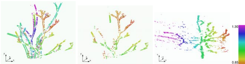
Fig. 14. Left: The stereo reconstruction of the twigs scene. There are some mismatches near the base of the twigs and along the branch receding in depth. The reconstruction is not affected by those areas where there is failure of the ordering constraint. Middle: A cropping plane 1.03m from the cyclopean point was placed to highlight the twigs in the foreground. Right: A birdseye view of the reconstructed scene. The twigs are arranged in roughly three layers as can be seen by fusing the stereo pair.
