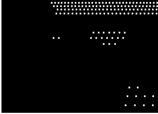
Figure 5. Mahalanobis distance transformed back to image plane. Blobs are positioned at the centers of windows used in segmentation. Brightness of the blob corresponds to the likelihood of object being present in the window.
