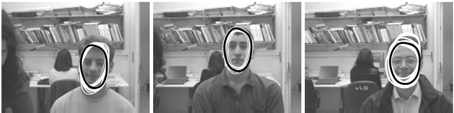
Fig. 12. Generalisation of face detection. Training on a single face generates a model that is still specific enough to discriminate each of a variety of faces against general scene background.
