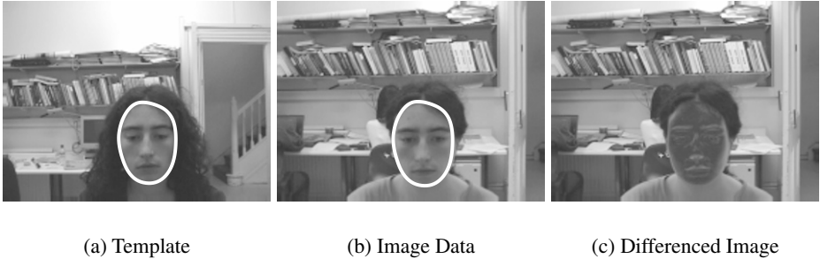
Fig. 5. Template subtraction. (a) The white contour marks the outline of the intensity template \bar{I} . When subtracted from an image I (b), the residue (c) is relatively small, as indicated by the dark area over the face.
