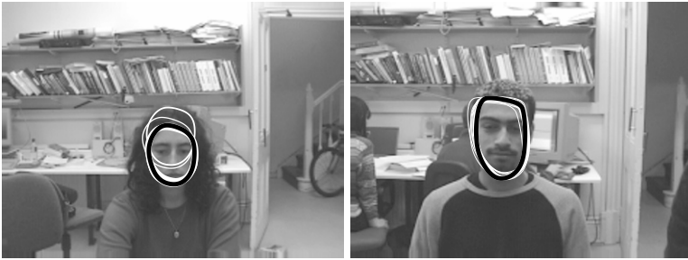
Fig. 11. Layered sampling demonstrated for individuals, using individual-specific models this figure. The prior for the position in the face is uniform in the x, y -translation over the image. The search takes place over two scales ( r = 20, 10 ) implemented via layered sampling, using 1500 samples in each layer.
