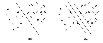
**Fig. 1.** Separating hyperplane and optimal separating hyperplane. Both solid lines in (a) and (b) separate the two identical sets described by circles and triangles. But the solid line in (b) leaves the closest points (filled circles and triangles) at the maximum distance. The distance between dashed lines in (b) gives the maximum margin.
