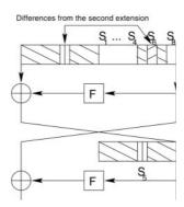
Fig. 3. The first two rounds in the third attack. The inputs to the S-boxes 1,2,3,4, and 8 in the first round are fixed.
