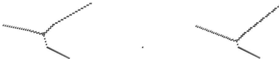
Fig. 4. From left to right, the set of CMGDs for the DT of the surface shown in Fig. 3, top, using DT^6 , DT^{26} , and 3 – 4 – 5 DT, respectively
