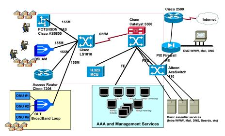
Fig. 2. Aveiro Digital City's Network Diagram
