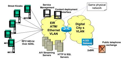
Fig. 9. Project 'EIRÓ' network architecture
