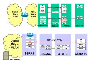
Fig. 3. Diagram of ADSL access scenarios. a) Access using RFC1483 bridged b) Access using PPP/PPPoA
