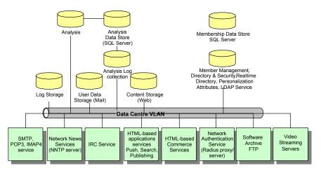
Fig. 8. Data Centre Service Architecture
