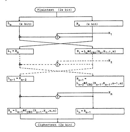
In contrast to the DES C80 does not use S-boxes, permutations or any other tables of fixed sizes.
