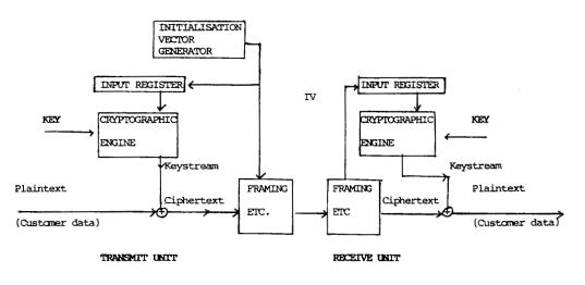
Figure 3 Encryption functions of the channel unit
