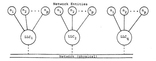
Fig. 9 Structuring of Network Entities and Addresses
