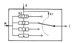
A second example is depicted in figure 5, where the set of mixing functions consists of functions on the message blocks only, followed by a modulo 2 addition. As a specific set of message block functions cyclic shifts of the message blocks are chosen. Assuming that the active eavesdropper uses modulo 2 addition it can easily be seen that he has to guess the number cyclic shifts of the message block difference correctly.
