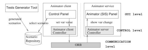
Fig. 3. Tool architecture
