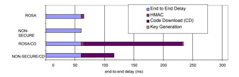
Figure 3. Comparison of end-to-end delay.
