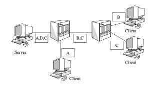
Fig. 4. Processing of a packet with multiple addresses.
