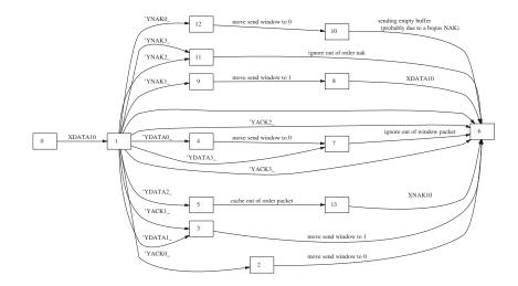
Fig. 4. Behavior of I-protocol when sending 1 data packet, and receiving a reply.
