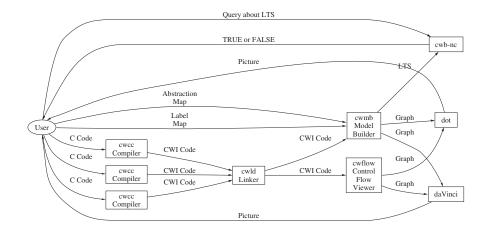
Fig. 2. System architecture at the executable-component level.
