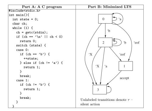
**Fig. 1.** A simple C program to recognize  $a^*b^*$  and its minimized LTS
