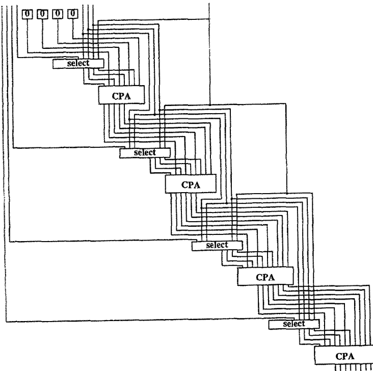
Figure 10. The abstract sketch of the mult : ((y_4 y_3 y_2 y_1), (x_4 x_3 x_2 x_1)) .
